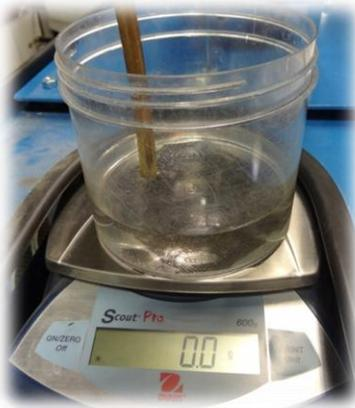
Water jacket and cylinder are filled. Scale is zero'd
