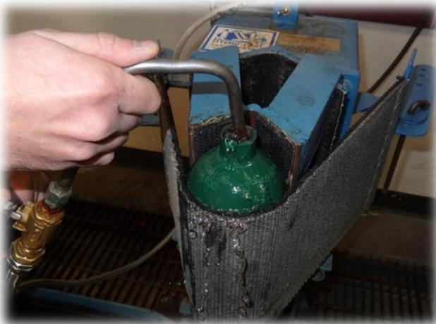
Cylinder is placed in vise & filled with water
