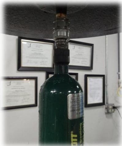
Cylinder is attached to water jacket lid
